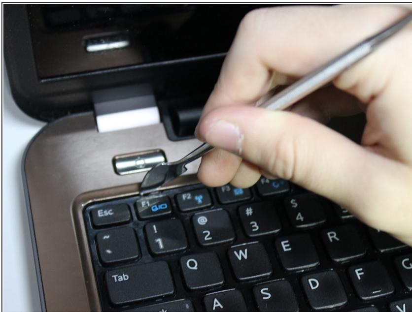
**⚠** A metal spudger can scratch delicate internal parts. Be extra careful when removing the keyboard.
