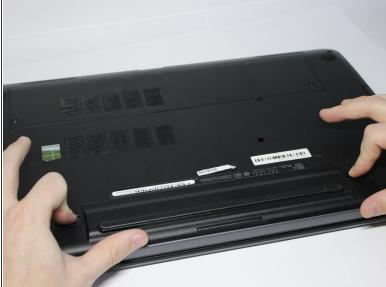
Slide each latch away from the battery to unlock it.
