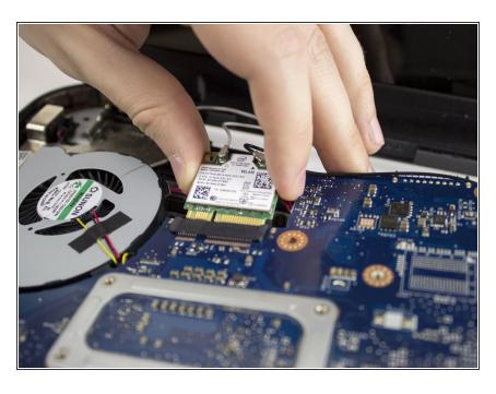
Remove the Wi-Fi chip by pulling upwards.
