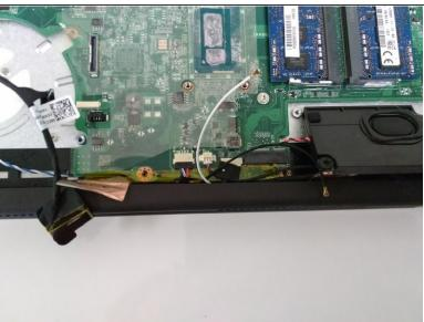
Unhook the speaker cables from under the catch under the hinge.
