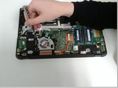
• Remove the two M2x2.5mm P0 Philips screws from the fan.
