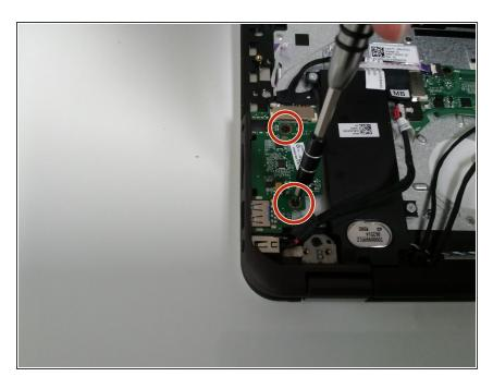
Remove the M2x2.5mm P0 Philips screw from the USB controller.
