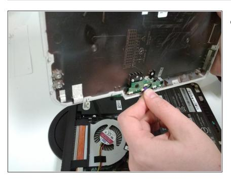
Unlatch the LED indicator from the back panel.
