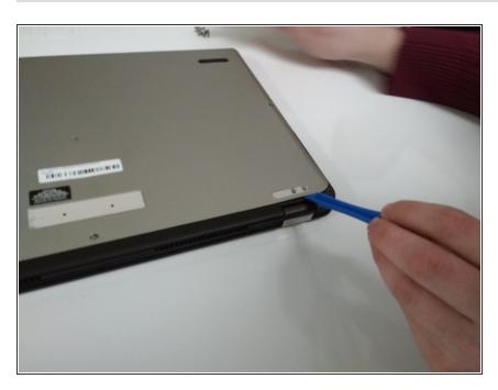
Near the hinges, wedge a plastic opening tool under the back panel.
