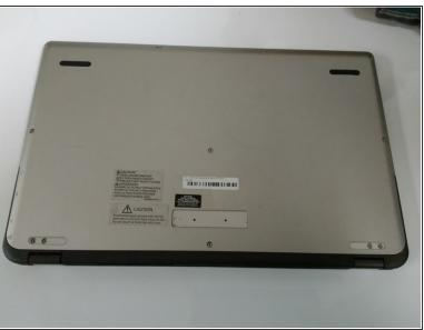
Using the plastic opening tool, remove the two rubber feet closest to the hinge.
