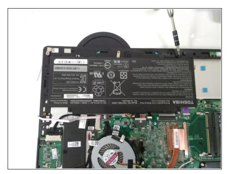
Using a P0 Philips head screwdriver, Remove the four M2x2.5mm P0 Philips screws from the battery.
