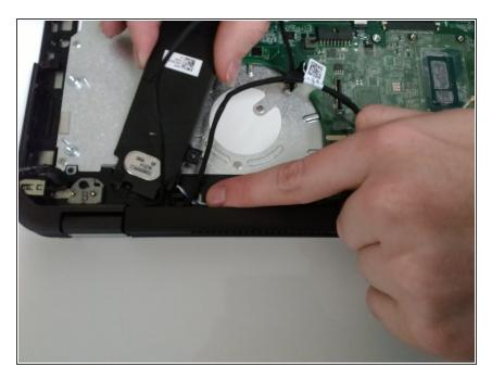
Unhook the speaker from under the hinge cable mounts.
