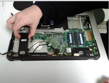
Remove the two M2x4mm PH0 Philips screws for the speaker mounts.
