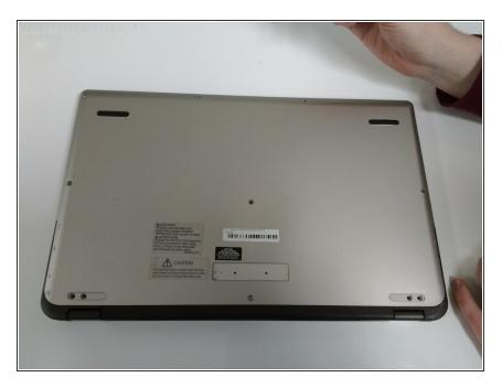
Remove the 12 M2x4mm PH0 Philips screws.
