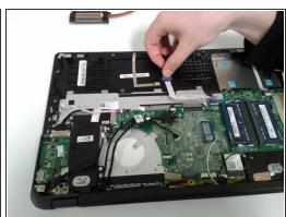
Disconnect the ribbon cable of the touchpad from the motherboard.
