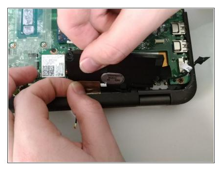
Remove the copper tape from the speaker cord.
