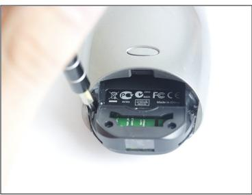
• Locate and unscrew the four 50mm screws using the Philips #0 screwdriver.
