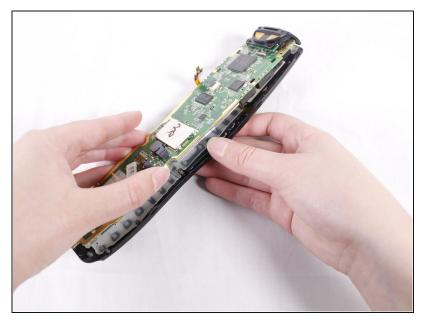
Using your hands, carefully separate the motherboard from the rest of the remote.
