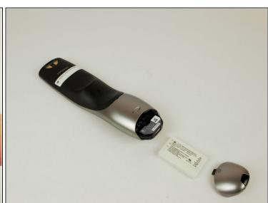
• Push the battery in, pull it up, and slide it out.
