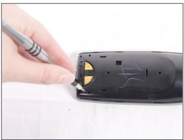
• Locate the three 50mm screws on the back of the remote and remove them using the Phillips #0 screwdriver.
