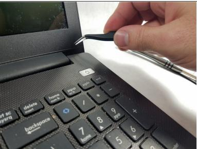
Using the tweezers, remove the 2 black plastic adhesive covers from the bottom corners of the screen frame.
