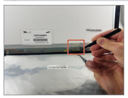
Using the <u>tweezers</u>, peel back the tape securing the screen wire to the laptop.
