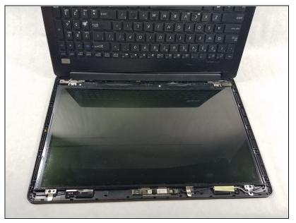
Flip the laptop around and lay the screen flat on your work space with the laptop hinge away from you and the keyboard assembly standing vertical.
