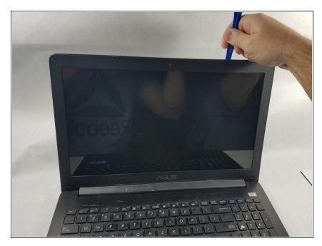
Using the plastic opening tool, pry the screen frame away from the screen.
