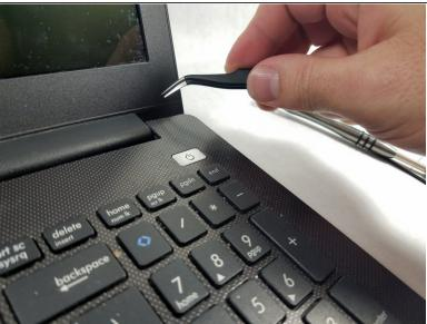
Using the tweezers, remove the 2 black plastic adhesive covers from the bottom corners of the screen frame.
