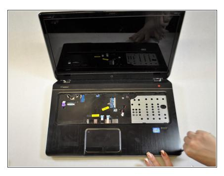
• Pry open the top panel of the laptop with a metal spudger.
