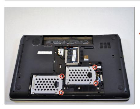
Remove the 2 Phillips PM2.5×5.5 top screws from brackets on both hard drives.
