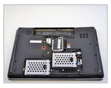
Remove the Phillips PM2.5×4.0 screw that attaches the optical drive to the laptop.
