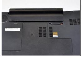
Slide the battery release latch to the left which is located on the right-hand side of the battery.
