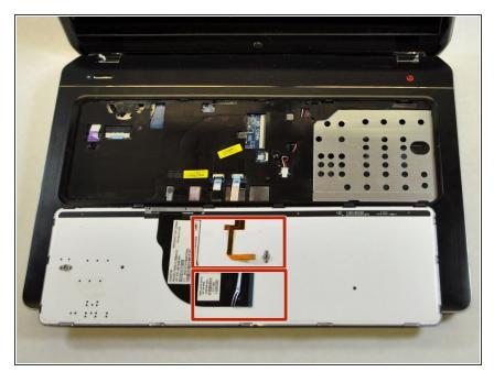
Release the connectors that attach the keyboard to the laptop.
