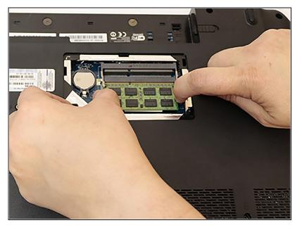
Push the two bottom tabs outwards and the bottom stick of RAM will pop up. Gently remove the bottom stick of RAM by pulling it out.
