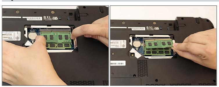
• Push the two top tabs outwards and the top stick of RAM will pop up. Gently remove the stick of RAM by pulling it out.
