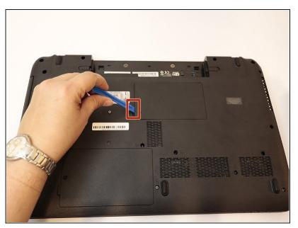
Use the plastic opening tool to pry open the RAM cover.
