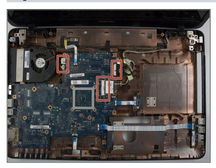
Disconnect the wire connectors by gently prying them apart with the flat end of the spudger. This can also be accomplished by gently wiggling the connector until it comes apart.
