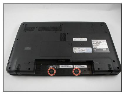
Remove the two screws from the underside of the laptop, where the battery was located, using the Phillips #1 screwdriver,
