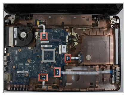
Disconnect the wire ribbon cables by gently lifting up the clips with the spudger or gently lifting on the blue tabs until the clips release the ribbon cables.
