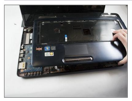
Remove the top plastic cover by lifting it from one of the corners. It should come off easily.
