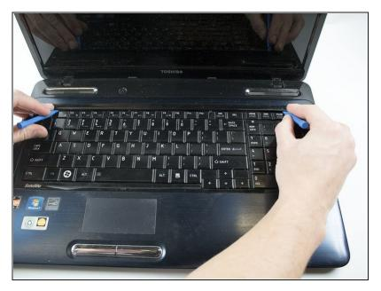
Pry up the thin narrow strip of facing above the keyboard using the opening tool.
