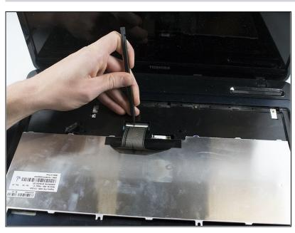
The ribbon is attached by a white clip. Wedge the white clip up carefully using the spudger. This will release the connector ribbon and you can now remove the keyboard.
