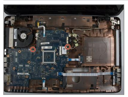
Remove the two screws using the Phillips #1 screwdriver.
