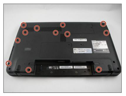
Remove the twelve screws from the underside of the laptop using the Phillips #1 screwdriver.
