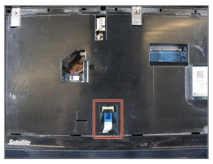
Detach the ribbon cable with black clip by carefully using the spudger tool and prying up the black clip gently or gently lift up on the blue tab until the clip releases the ribbon cable.
