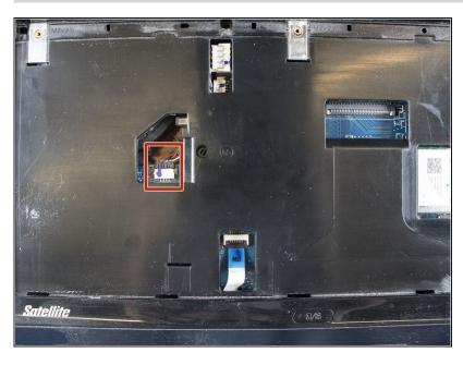
Detach the wire connector by using the flat side of the spudger tool to pry the connector apart; this can also be accomplished by gently wiggling the connector until it comes apart.
