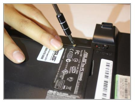
Unscrew the 2 screws on the CPU/Access panel on the back of the device
