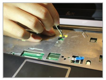
Unscrew the 8 screws on the back chassis and the 7 screws on the keyboard area
