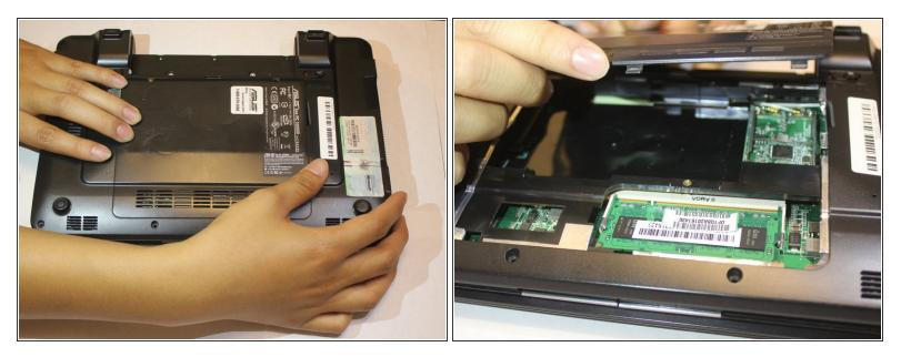
• Ensure all screws in the battery area are unscrewed and lift access panel
