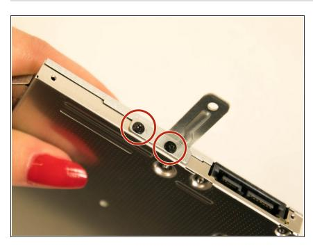
If you need to replace the bracket on the Optical drive, remove the two Phillips #0 screws holding the bracket in place. The bracket can be placed on the new drive. To reassemble your device, follow these instructions in reverse order.
