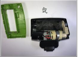
Remove the four 13.0 mm Phillips #0 screws and remove the green cover.
