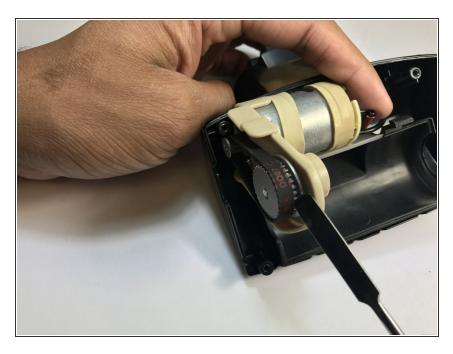
Take the belt off the gear by using a spudger.
