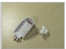
Use a spudger to pry the gear housing unit from the base.
