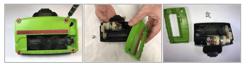
• Remove the four 13.0 mm Phillips #0 screws and remove the green cover.
