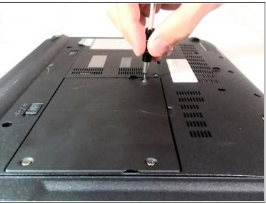
Unscrew the three screws on the hard drive panel using a Phillips Head #00 screwdriver.
