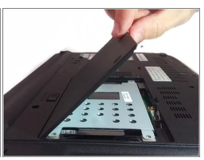
Lift the hard drive panel up from the small cut out at the bottom with your finger to expose the hard drive.
