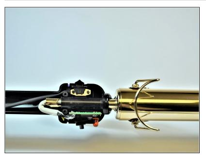
Once the screws have been removed, set them aside and with a pry tool, firmly pull the handle body apart in half lengthwise.
