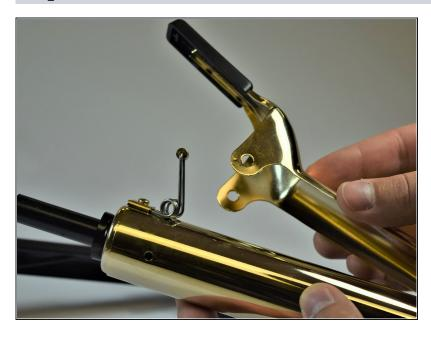
Once both screws have been removed, continue to remove the top clamping half of the mechanism from the body of the Iron.
