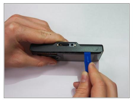
Take the iFixit opening tool and place it between the crevice as shown.
