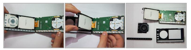
• Once the screws have been removed, the motherboard is free to come out.
