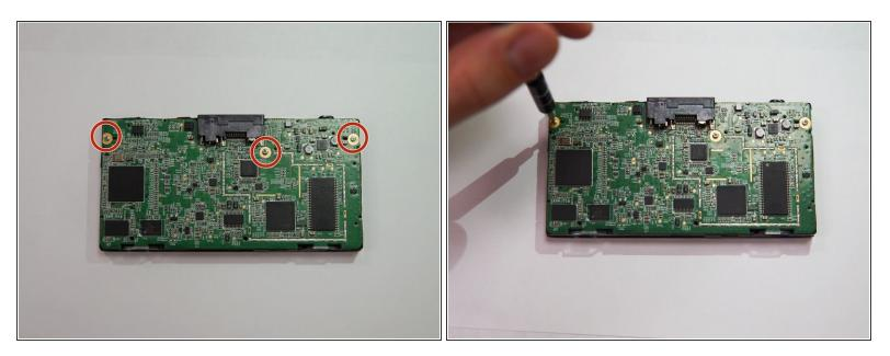
Use the Phillips PH00 to remove the three marked screws.
