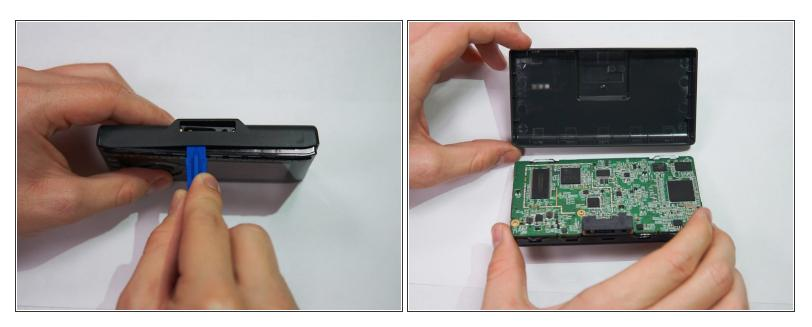
• Apply pressure to the iFixit opening tool, pushing down until the the plastic casing pops off.
