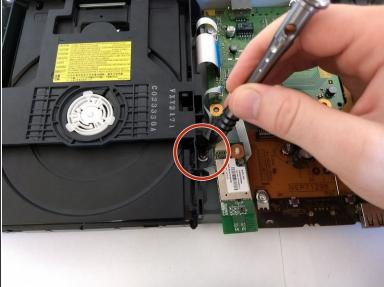
Remove screws surrounding disk drive that attach it to outer cover.
