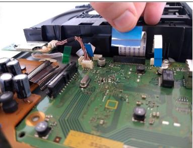
Remove the one green andthree blue tabs pictured that connect the disk drive to the board. Try to do so carefully, to avoid damage to the hardware.
