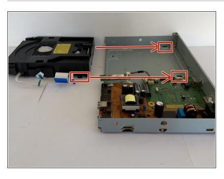
Carefully take the drive out of the device. Note where the feet need to go back in for reassembly. To reassemble your device, follow these instructions in reverse order. Ensure the feet of the disk drive go back in the holes.
