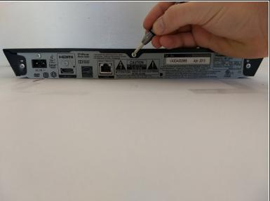
Using a Phillips #1 screwdriver, unscrew the back three screws.
