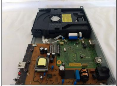
Pull the module board straight up, removing completely. The second photo is how your device should look with the WiFi board removed.
