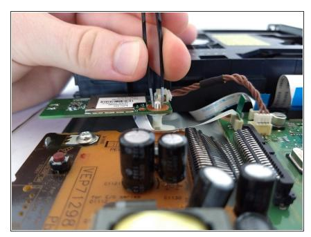
Using tweezer, compress the white knob holding the wifi module board in place.
