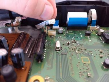
Locate reddish brown cable. Detach from green circuit board by pulling upward.
