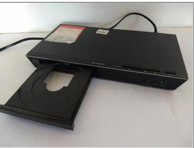
First, before powering off, press the eject button to open the tray.
