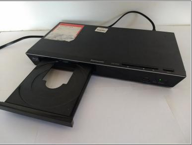
First, before powering off, press the eject button to open the tray.
