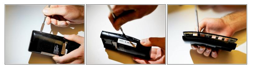
• Carefully wedge the flat metal spudger between the two sides of the remote until they separate. An intermediate amount of force will be needed to separate the pieces.
