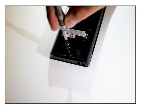
Use a TA20 screwdriver to remove the screw in the center of the battery slot.
