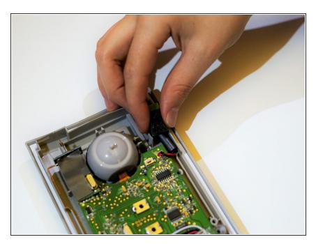
Carefully remove the microphone from the casing by pulling away from the device.
