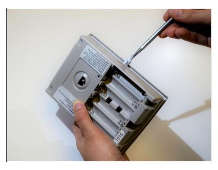
Use the spudger to separate the top and bottom halves of the screen.
