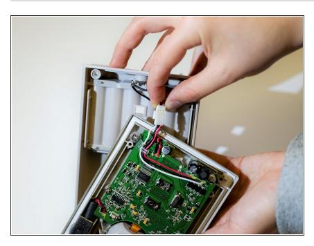
Disconnect the wires from the green motherboard to the bottom half by pulling apart the connecting pins.
