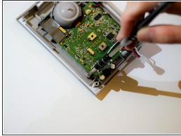
Unscrew all 3 Phillips head screws on the outside edges of the motherboard.
