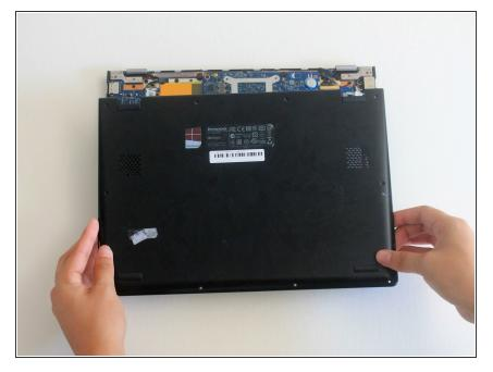
Now that the screws are removed, gently lift the back panel upwards to detach it from the rest of your laptop.
