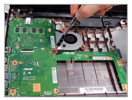
Using the J00 screw bit in the iFixit tool kit, remove the three screws securing the fan to the case. One screw connected to the bottom case (4cm), one connected to the motherboard (4cm), and one screw connected to the Wireless Card (5cm).
