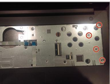
Using the Phillips J0 screwdriver, remove the ten screws shown.
