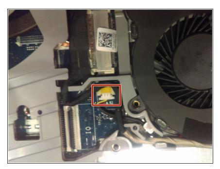
Remove the fan cable, indicated by the red marker in the picture, by pulling it out from the connector. Be careful to pull it out by the plastic end instead of by the cable.
