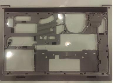
Flip the laptop to the back. Remove the wire indicated by puling directly to the left and pressing the cream colored bases, then use the metal spudger to pry off the case.
