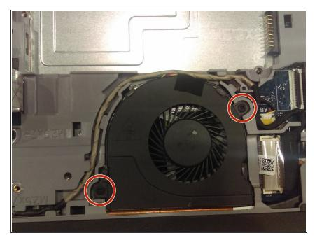
After you have removed the ribbon cable, locate the screws indicated in the photo by the red markers (2 in total) and remove them with a Phillips J0 screwdriver.
