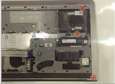
Using the Phillips J0 screwdriver, remove all the screws from the case. There is a total of 16 screws. CAUTION: The bottom left screw does not remove from the laptop.
