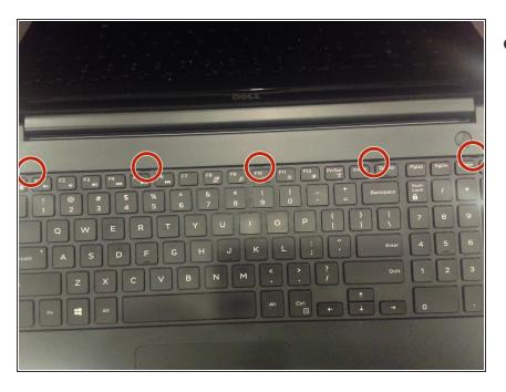
Using the metal spudger, press the five indicated tabs, then run the spudger around the left and right sides of the keyboard. The keyboard can then be removed by pulling it up and towards the screen. Do not pull it very far, as there are still cables connected to it.
