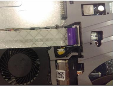
Start by removing the white ribbon cable. Lift up the black tab indicated by the red marker to disconnect the ribbon cable from the connector. Be careful while removing the ribbon cable, as it will possibly be taped to the fan.
