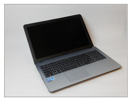
Power down the laptop using the device's power button in top right corner of the keyboard. Ensure that the device's power cord is disconnected.
