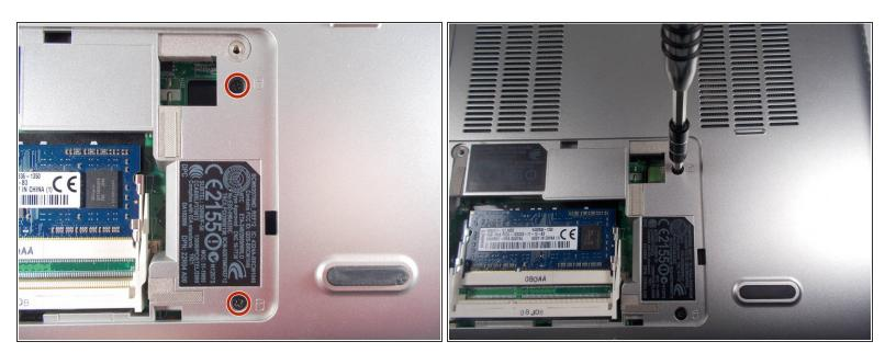
Use a JIS 1 screwdriver to remove (2) 2.5mm screws located on the right side of the RAM bay.
