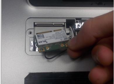
Remove the mini card as it flips upward.
