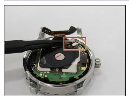
Utilize tweezers to pull the white battery connector from the motherboard.
