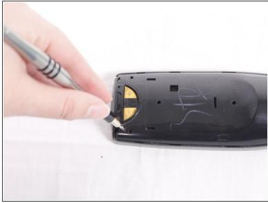
• Locate the three 50mm screws on the back of the remote and remove them using the Phillips #0 screwdriver.
