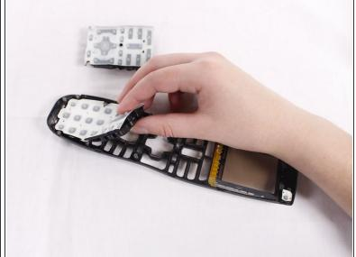
Peel off the button pads from the device frame.
