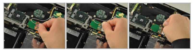
Detach the white and black wires from the Wi-Fi card, located in the central area of the laptop.
