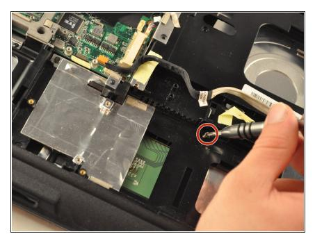
Using the PH1 screwdriver, remove the .75 mm screw from the plastic housing corner, located in the bottom-right corner of the laptop.
