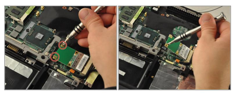
Using the PH 1 screwdriver, remove the two .25 mm screws from the Wi-Fi card.
