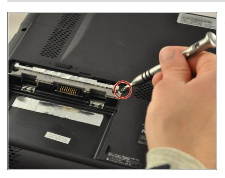
Remove the one .5 mm screw located in the top right corner of the battery compartment.
