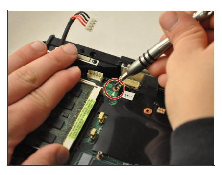
Using the PH 1 screwdriver, remove the .75 cm screw from the topmiddle section of the motherboard.
