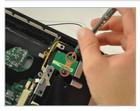
Using the PH 1 screwdriver, remove the two .5 mm screws from the RAM drive.
