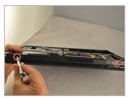
Using the PH1 screwdriver remove the two .75 mm screws from the hinge side of the laptop.
