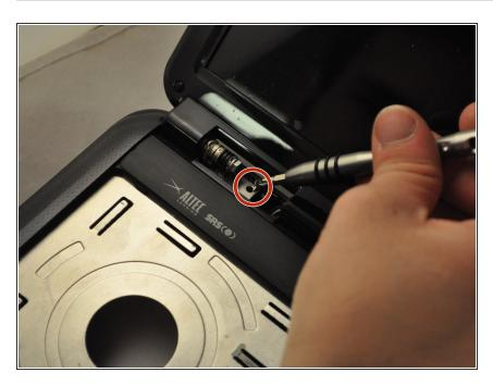
Use the PH1 screwdriver to remove the .75 mm screws from the hinges.
