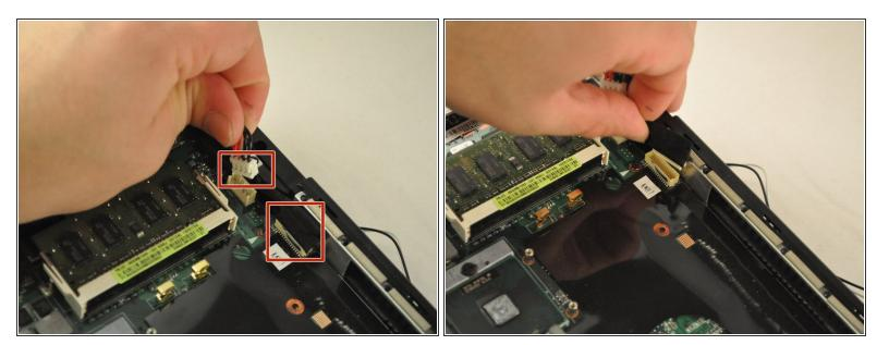
Unplug the wire and black cables on the motherboard, located in the upper-left corner of the laptop.
