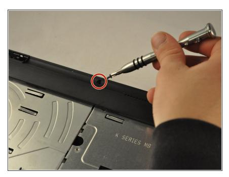
Using the PH1 screwdriver, remove the .75 mm screw from the bottommiddle section was previously covering.
