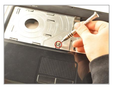
Using the PH 1 screwdriver, remove the .75 cm screw from the bottommiddle section where the keyboard was previously covering.
