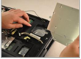
Slide the disc drive out of its slot.
