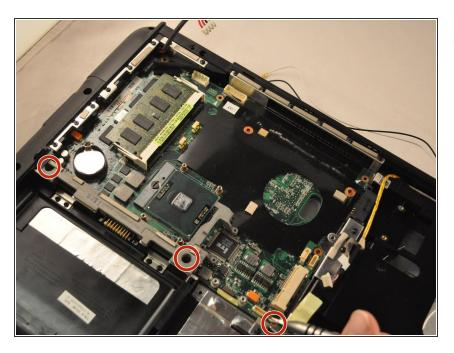
Using the PH1 screwdriver, remove the three .75 mm screws from the bottom corner of the motherboard.
