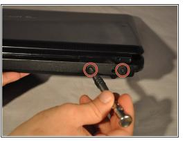
• Using the PH1 screwdriver, remove the four 4 .75 mm screws that are located on the vent panel.
