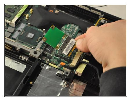
Slide the Wi-Fi card out of its slot to remove.
