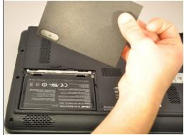
Lift the exposed lip and remove the battery cover.
