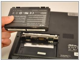
Press the tabs on the battery and lift them. The battery should come out easily.
