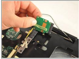
Slide and lift the RAMdrive out of its port.
