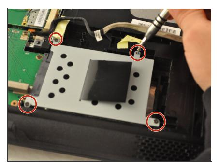
Using the PH1 screwdriver, remove four .75 mm screws from the driver, located in the bottom-right corner of the laptop.
