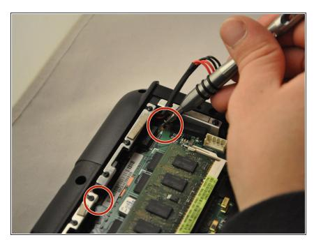
Using the PH1 screwdriver, unscrew the two .75 mm screws from the topleft corner of the motherboard.
