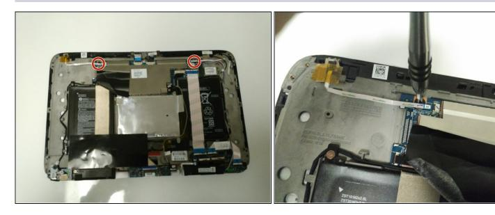
• Unscrew the two 2mm zero insertion force connectors. Slide aside the white wires to properly unscrew.
