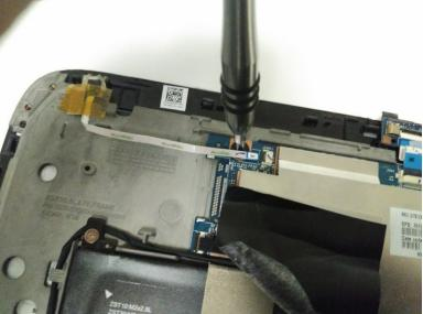
Unscrew the two 2mm zero insertion force connectors. Slide aside the white wires to properly unscrew.
