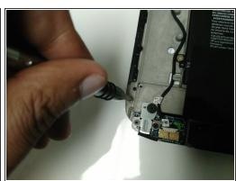
• Use the PH1 screwdriver to remove eleven 4mm Phillips screws.
