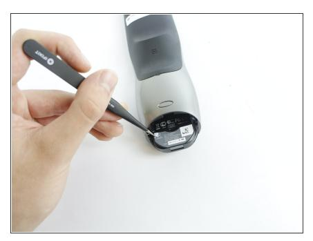
Using tweezers, peel off the sticker located under the battery cover to reveal two screws.
