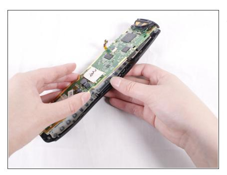
Using your hands, carefully separate the motherboard from the rest of the remote.
