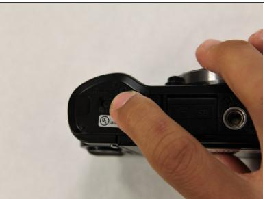
Slide the switch on the bottom of the battery flap to unlock it.
