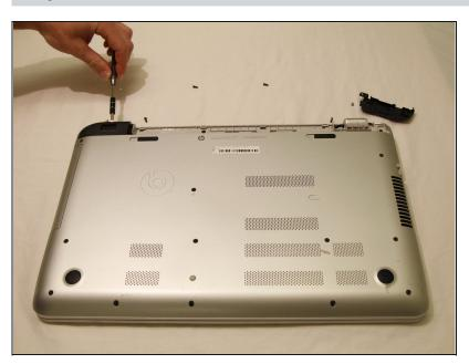
Use a plastic opening tool to pop the corners off by wedging between casing. Do this for both legs as depicted in the picture.
