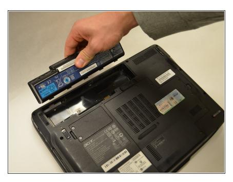
Grasp the inside edge of the battery and lift to fully detach the battery from the computer.
