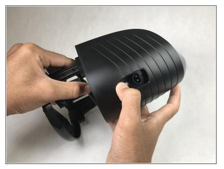
Press inward on the side charging port while pulling cover from the base to separate.
