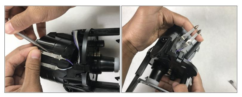
• Remove charging terminals by inserting a spudger from bottom the and sliding terminals up.
