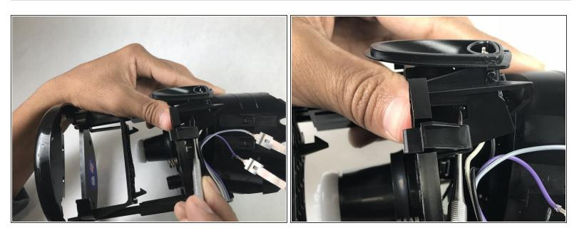
• Remove side charging port by prying tabs outward and rotating port upward.
