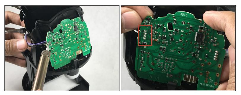
Remove solder from circuit board and remove charging harness.
