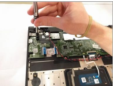
Using a JIS #0 screwdriver, unscrew the three 4mm screws securing the daughterboard in place.
