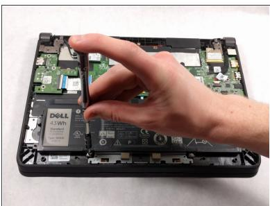
Using a JIS #0 screwdriver, unscrew the two 4mm screws securing the battery in place.
