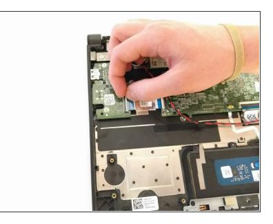
Disconnect the bridge connection ribbon cable from the motherboard.
