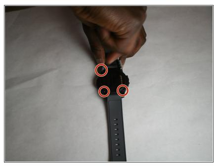
Remove 4 4.5mm Phillips head screws from back side of watch using PH00 Phillips head.
