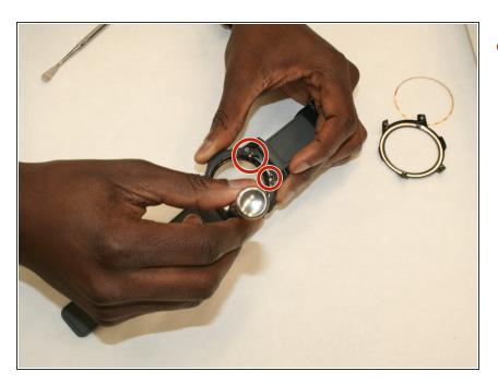
Remove 4 4.5mm Phillips gold screws from back of watch using PH00 Phillips head.
