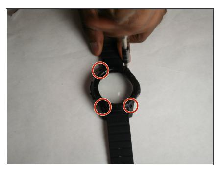
Remove 4 7.0mm hex-screws from front of watch using H1.5 Hex head.
