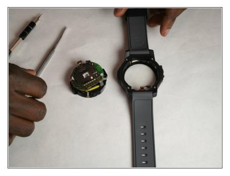
• Carefully remove motherboard & internal screen.
