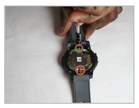
Remove 2 3.0mm Phillips screws from motherboard using PH00 Phillips head.
