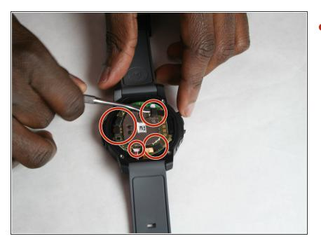
Unclip 5 latches from motherboard using a spudger.
