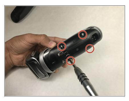
Use a Torx T8 to remove (4) 10 mm screws from housing.
