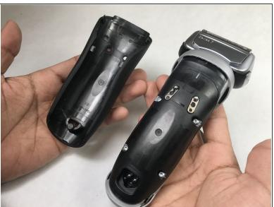
Use a spudger to remove the rubber piece on the back of the razor.
