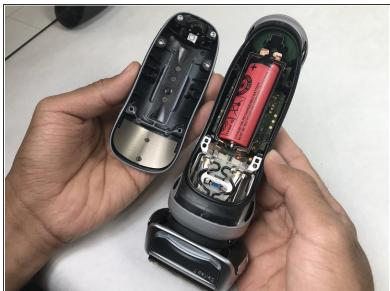
Remove the rear cover from the device.
