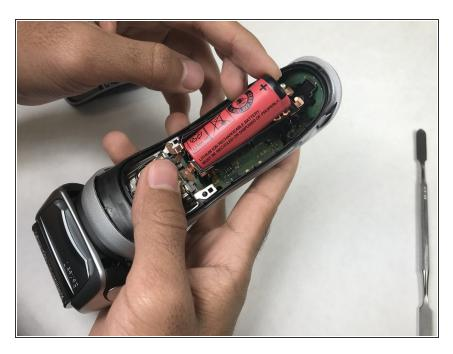
Remove the battery from the holster inside the device.
