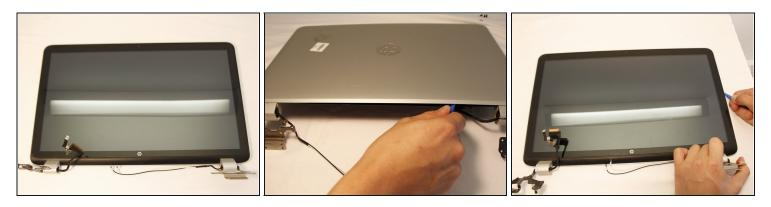
Use a plastic opening tool along the gap between the screen and the back panel to separate the two pieces.
