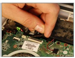
• With <u>tweezers</u> in hand, begin by disengaging the tab on the upper left corner of the motherboard. Using your fingers, disconnect the plug that is to the left of the tab.
