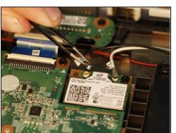
Using tweezers, gently remove the two cables connected to the WLAN module.
