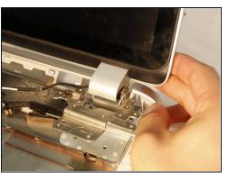
Remove the screen by pulling it forward from the casing. This allows the hinges to clear the casing.
