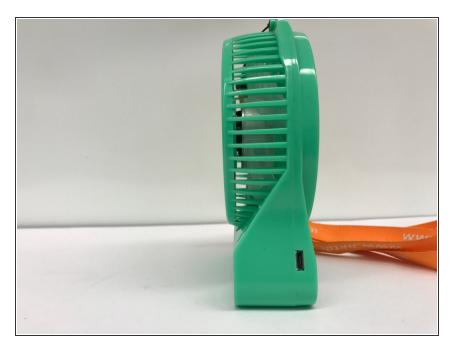
The side of the fan contains a micro-USB port through which the device receives it's charge.
