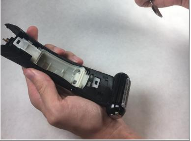
Use a nylon spudger to pry out battery pack and the attached LED board.
