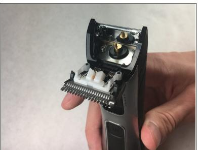
Place thumb behind trimming blade and push up to open.
