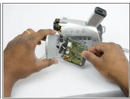
Now that all the screws are removed, use the plastic opening tool to gently pry the LCD monitor case open.
