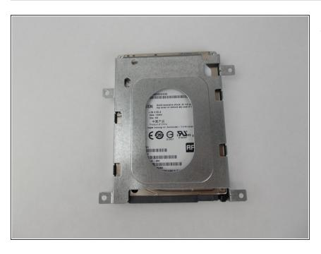
Remove screws from the metal plate enclosing hard drive and enclose replacement hard drive in metal plate.
