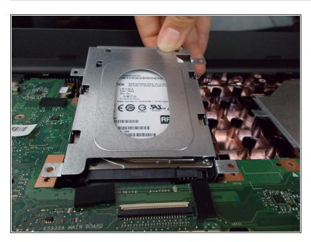
After all screws are removed, carefully disconnect the hard drive and slide it out.
