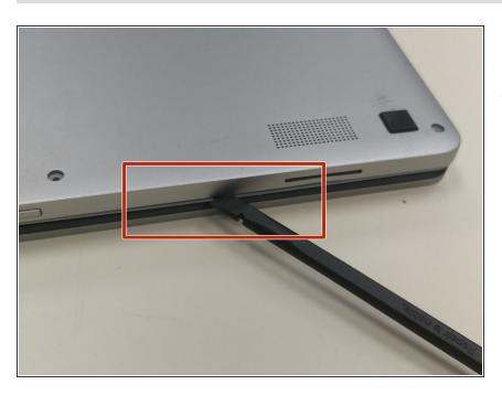
Using a plastic spudger, open the back cover and remove it from the laptop.
