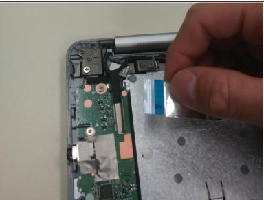
Find and remove the blue tape from the circuit board.
