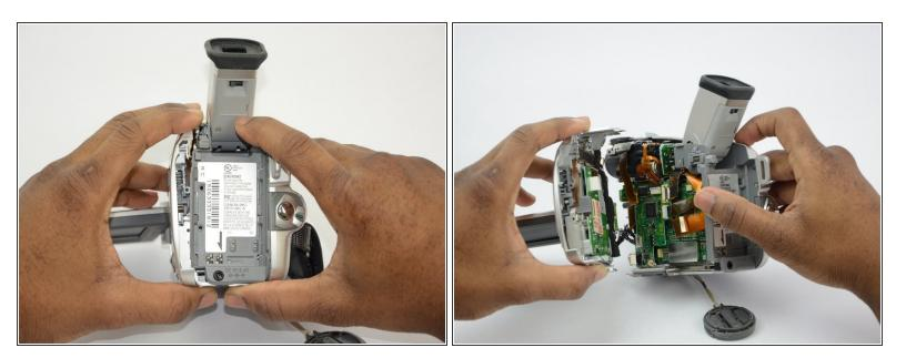
• Now that all of the screws are removed, gently pull off the side panel of the camcorder.
