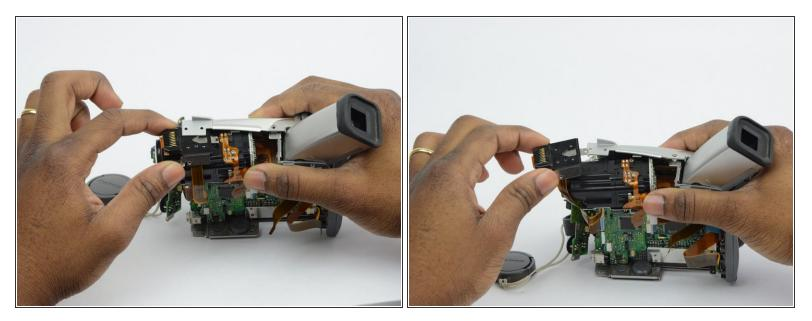
• Remove the final black metal plate that is holding the lens in place.
