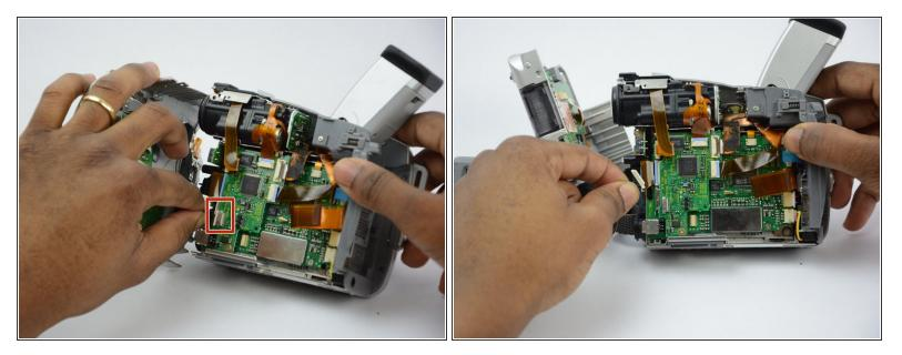
Gently pull the two black wires from their connections. These black wires are the only thing left connecting the side panel to the main body of the camcorder.
