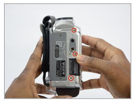
Remove all 3.75 mm screws from the bottom of the camcorder.
