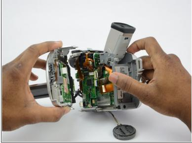
Now that all of the screws are removed, gently pull off the side panel of the camcorder.
