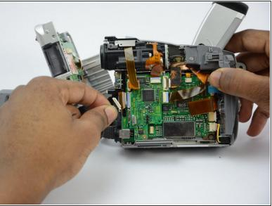
Gently pull the two black wires from their connections. These black wires are the only thing left connecting the side panel to the main body of the camcorder.
